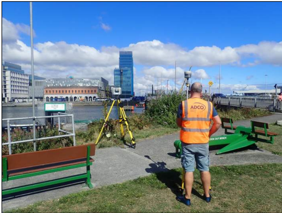
Plate 5: North-facing working shot of Laser-scan and GNSS survey in progress.
