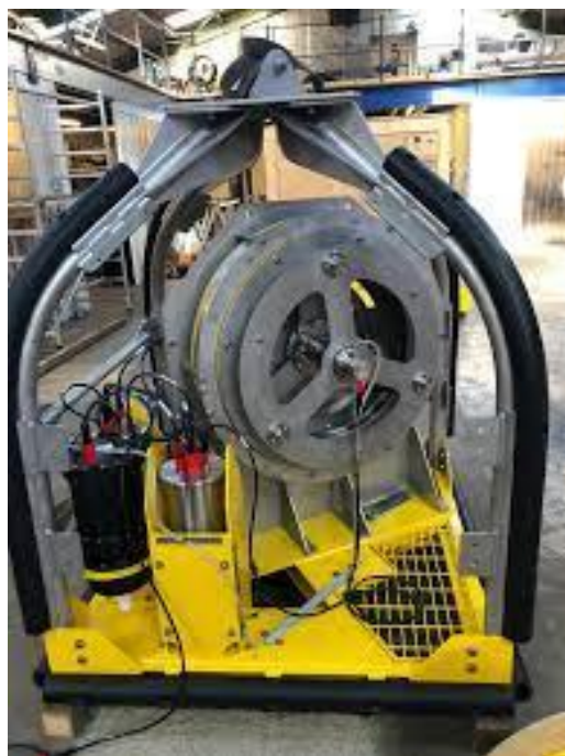
Figure 17: Neptune 3000 CPT Rig
