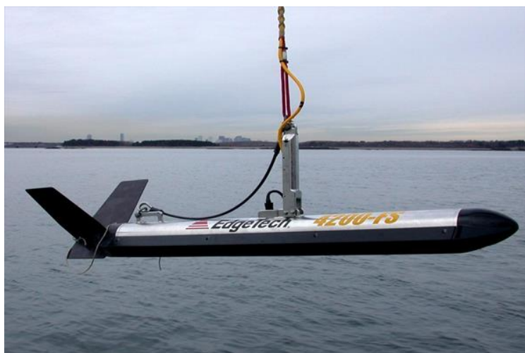
Figure 14: Deployment of Edgetech 4200 Tow fish
