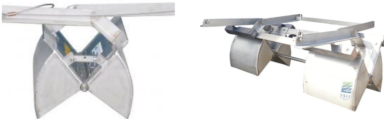
Figure 20: Single and Double Van Veen Grab
