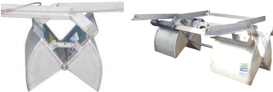
Figure 28. Single and Double Van Veen Grab.
