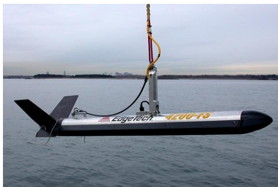
Figure 21. Deployment of Edgetech 4200 Tow fish.
