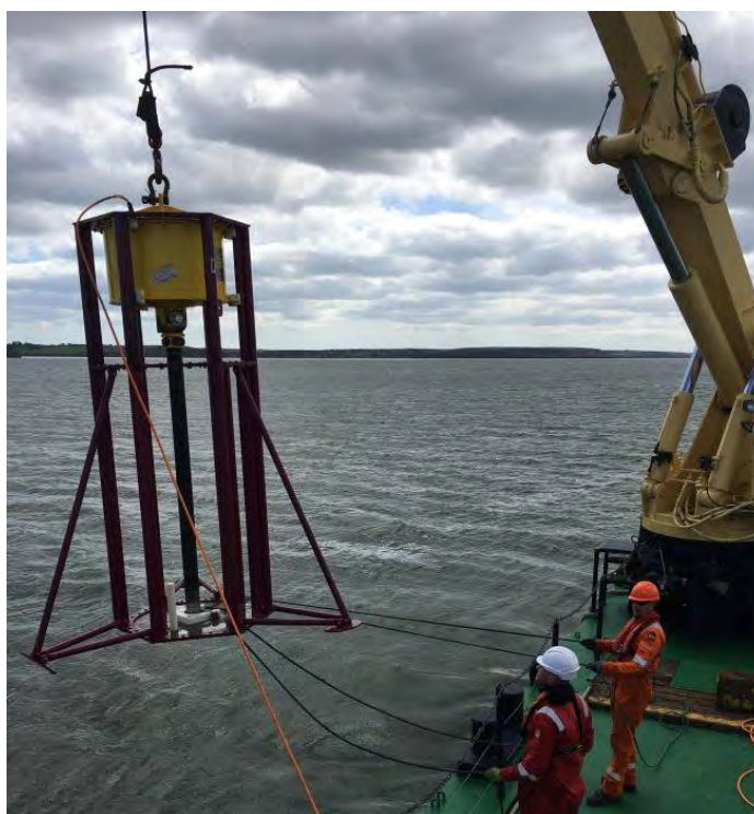
Figure 27. Deployment of Vibrocorer from Survey Vessel
