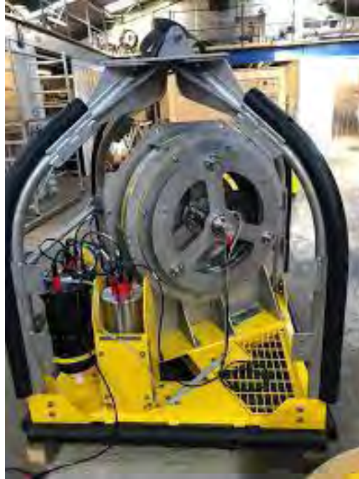
Figure 25. Neptune 3000 CPT rig
