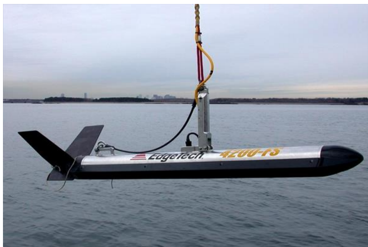
Figure 21. Deployment of Edgetech 4200 Tow fish.
