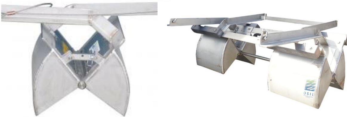
Figure 28. Single and Double Van Veen Grab.
