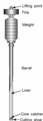
Figure 26. Gravity Corer schematic
