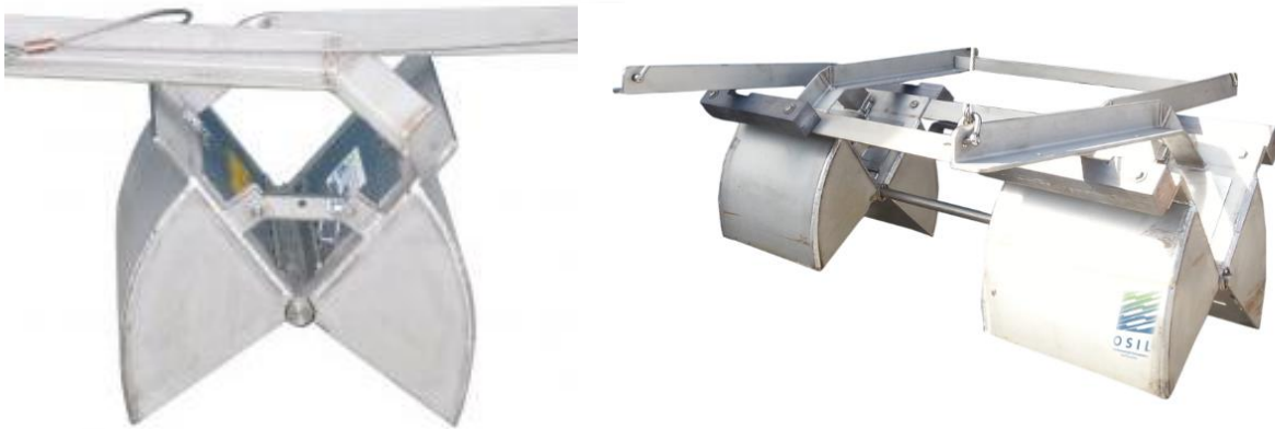
Figure 28. Single and Double Van Veen Grab.
