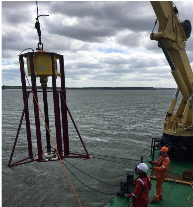
Figure 27. Deployment of Vibrocorer from Survey Vessel.
