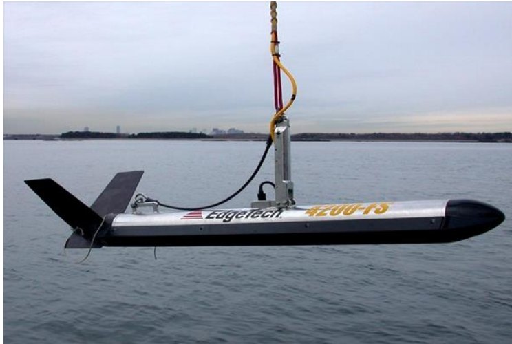
Figure 21. Deployment of Edgetech 4200 Tow fish.
