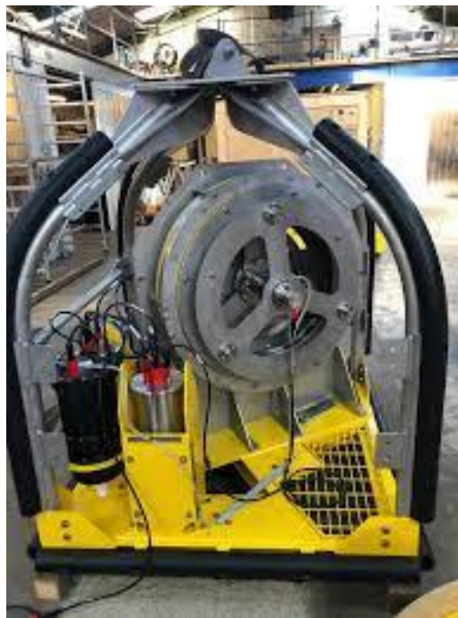
Figure 25. Neptune 3000 CPT rig.
