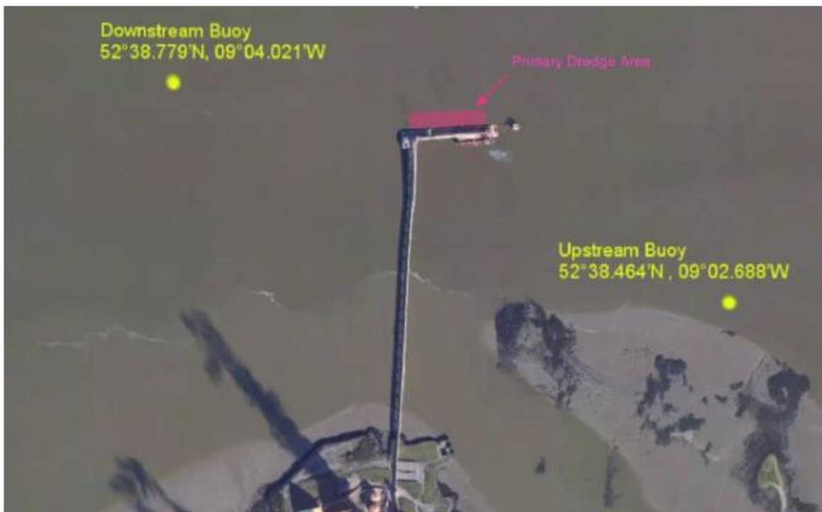
Figure 10-1: Location of the proposed suspended solids monitoring points
