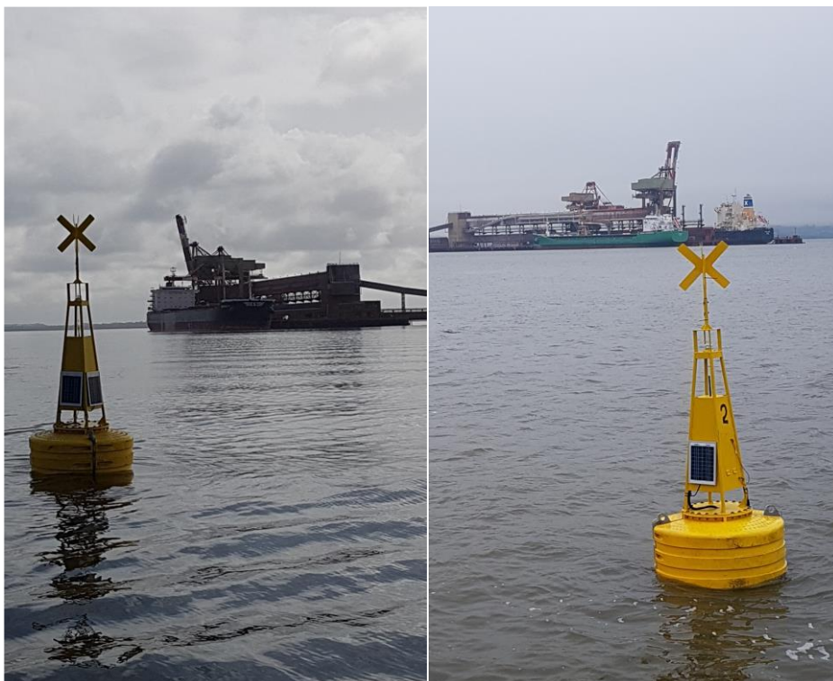
Figure 1 – IDS DB150 Data buoys similar to those deployed at Aughinish (downstream left, Upstream right)
