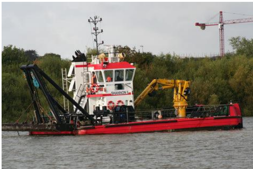
Figure 9. Plough dredger used in the Shannon Estuary M.V. Shannon 1©Irish Waterway History
