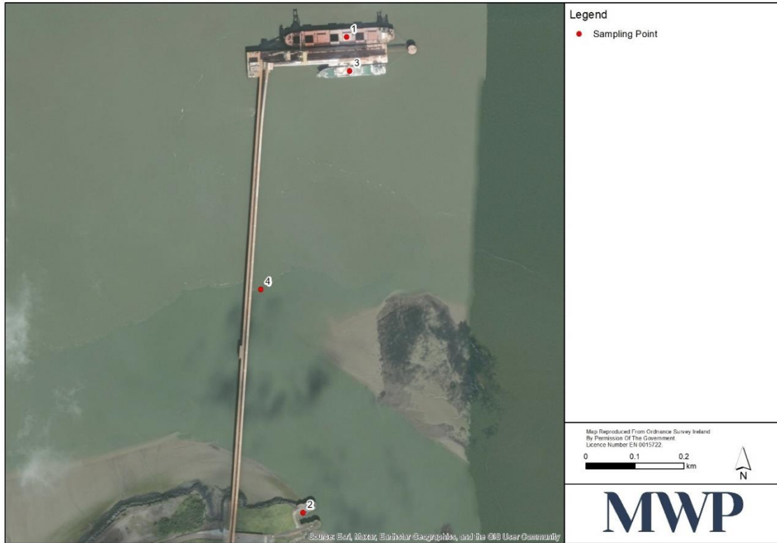
Figure 2-5: Location of the sediment sampling points for the chemical and granular analysis around the AAL Jetty.
