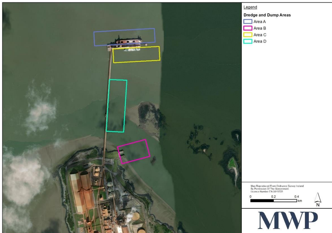
Figure 2-3 The proposed four dredge/dump sites around the AAL jetty.
