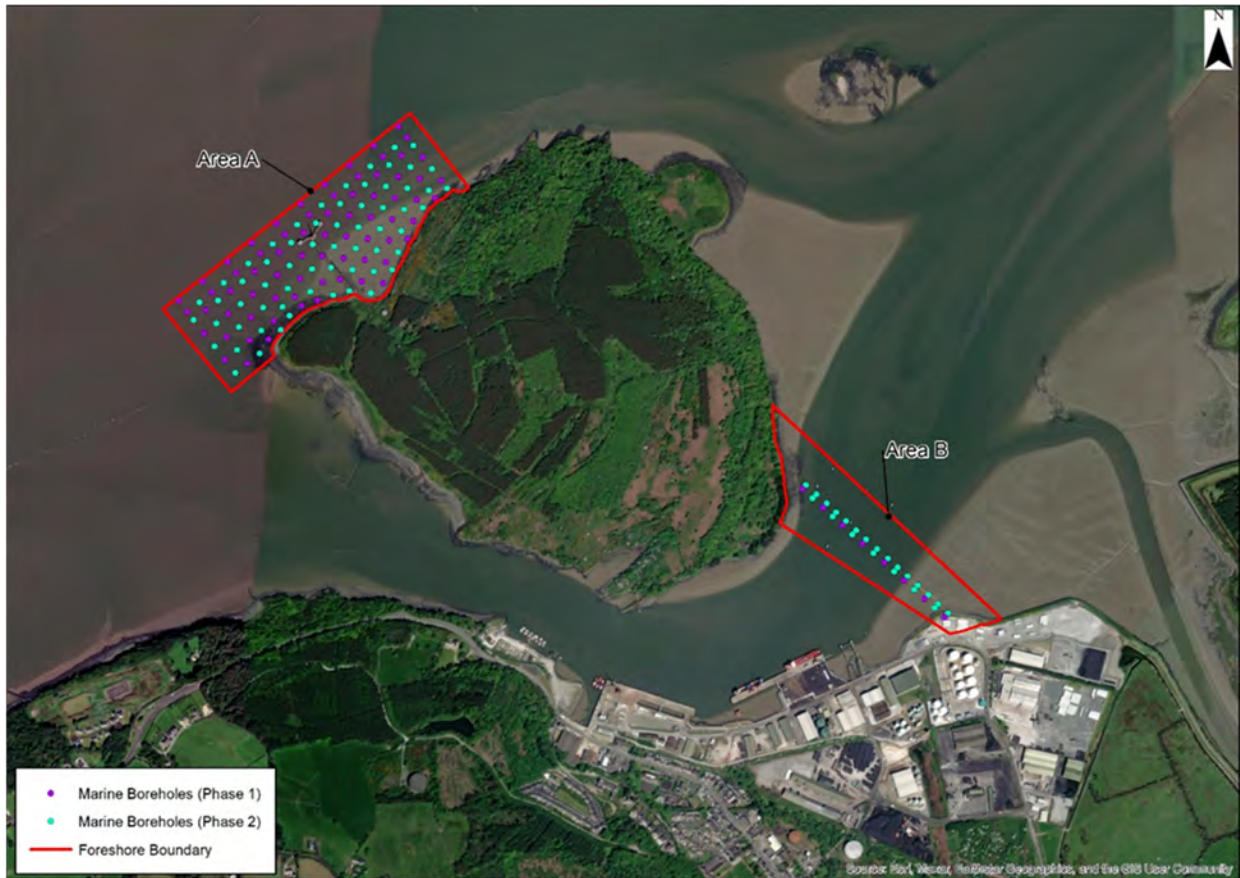
Figure 2: Proposed Site Investigations around Foynes Island, Co Limerick (geophysical surveys to occur within the red line boundary)
