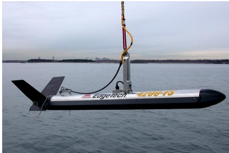
Figure 11. Deployment of Edgetech 4200 Tow fish.
