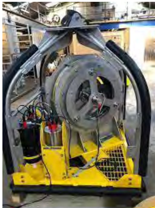
Figure 8. Neptune 3000 CPT rig
