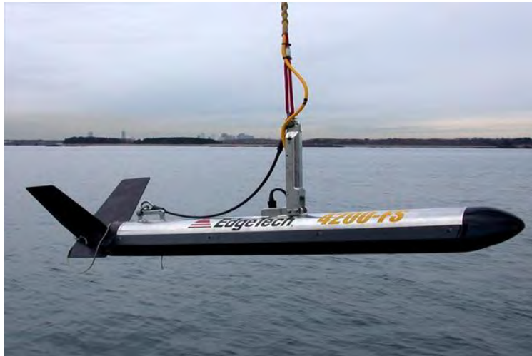
Figure 11. Deployment of Edgetech 4200 Tow fish
