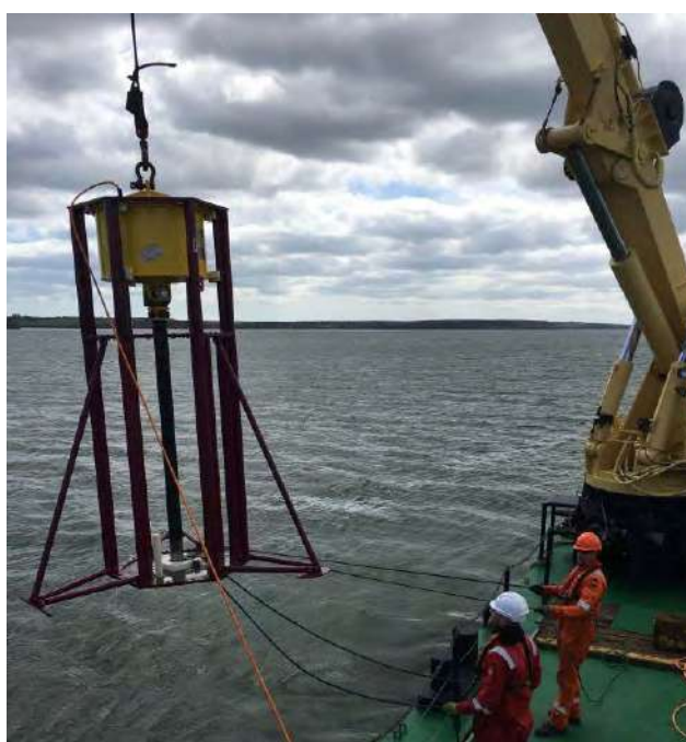
Figure 10. Deployment of Vibrocorer from Survey Vessel
