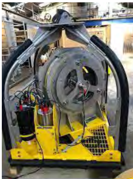
Figure 8. Neptune 3000 CPT rig
