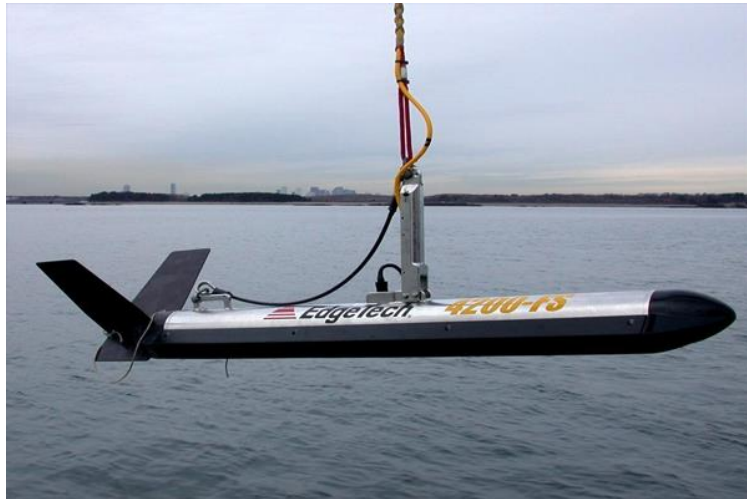
Figure 10. Deployment of Edgetech 4200 Tow fish.
