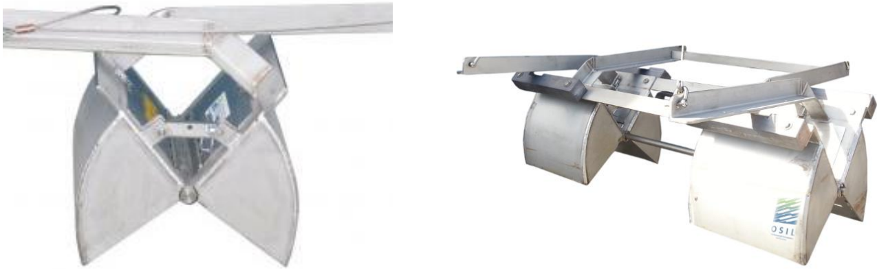
Figure 17. Single and Double Van Veen Grab
