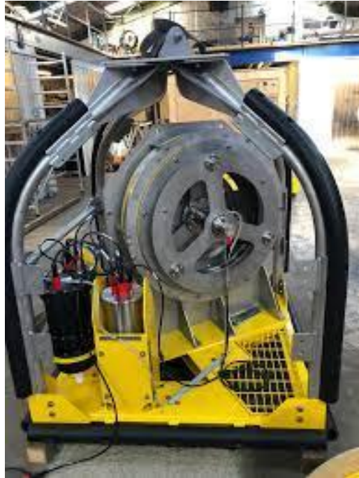
Figure 14 Neptune 3000 CPT rig.
