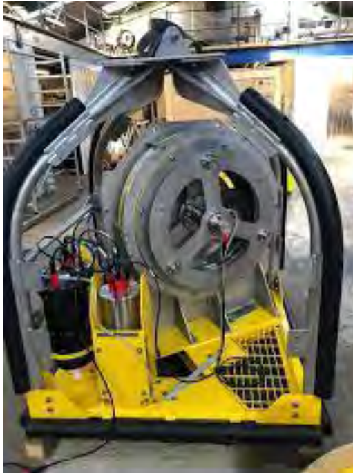
Figure 14 Neptune 3000 CPT rig.
