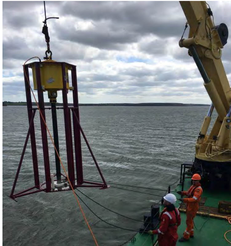
Figure 16. Deployment of Vibrocorer from Survey Vessel
