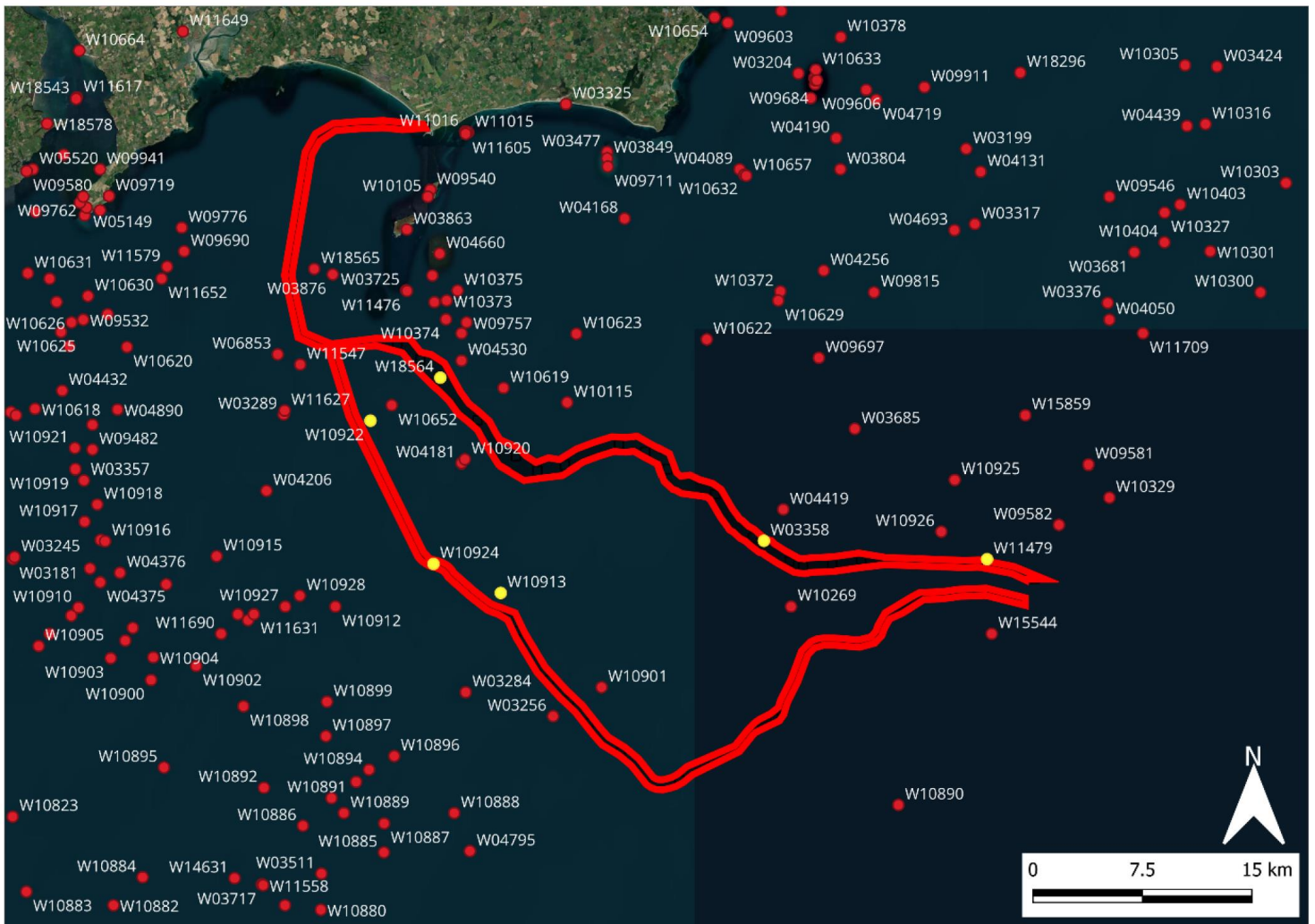
Figure 5. Proposed survey route with surrounding shipwrecks with known locations in the WIID. Wrecks within the corridor and within c. 100m are highlighted in yellow.
