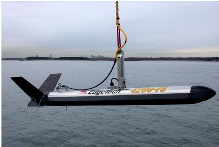
Figure 10. Deployment of Edgetech 4200 Tow fish.
