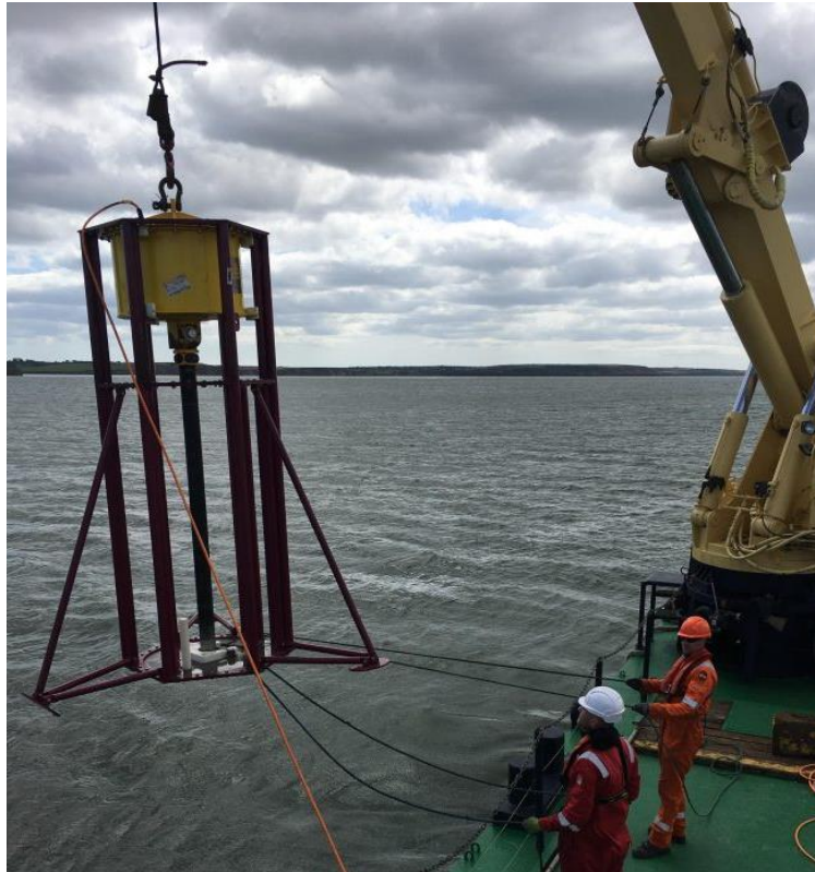
Figure 16. Deployment of Vibrocorer from Survey Vessel.
