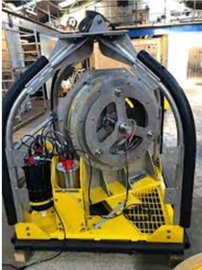
Figure 15. Neptune 3000 CPT rig.
