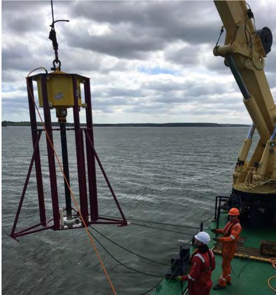
Figure 17. Deployment of Vibrocorer from Survey Vessel.
