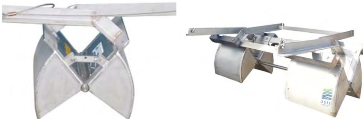
Figure 18. Single and Double Van Veen Grab.
