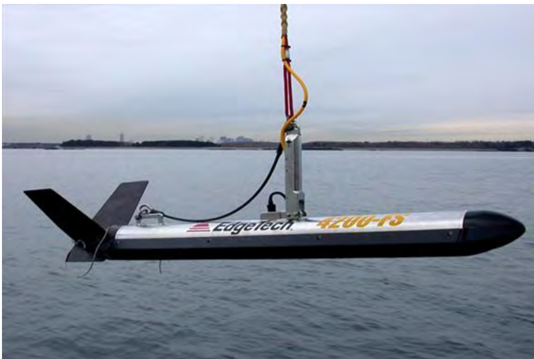
Figure 11. Deployment of Edgetech 4200 Tow fish
