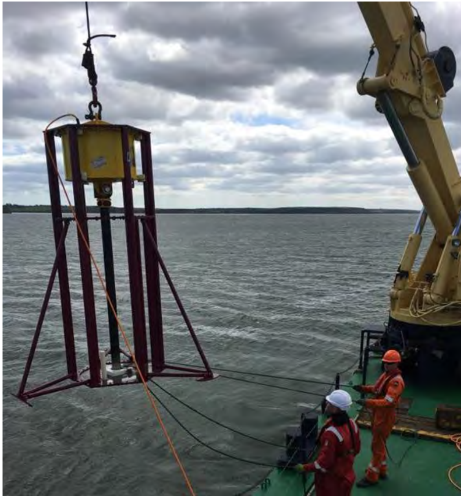
Figure 17. Deployment of Vibrocorer from Survey Vessel.
