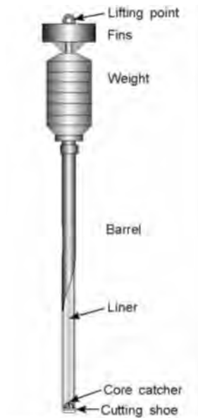
Figure 16. Gravity Corer schematic.
