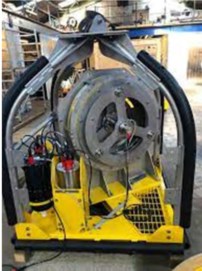
Figure 15. Neptune 3000 CPT rig.
