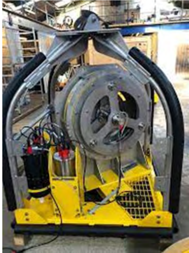
Figure 15. Neptune 3000 CPT rig.
