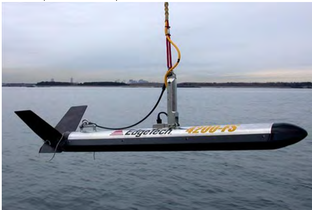
Figure 11. Deployment of Edgetech 4200 Tow fish
