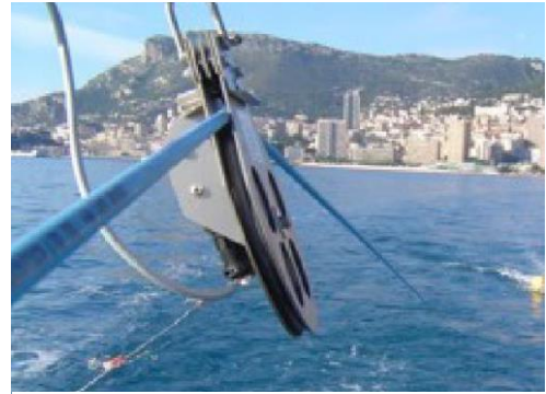
Figure 2.5 Counting pulley for winch-towed C-Max CM2 SSS
