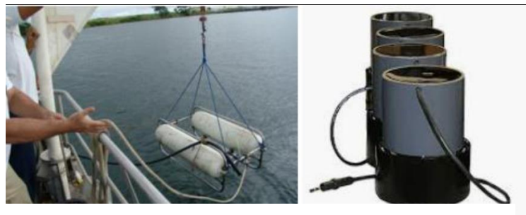
Figure 2.6 Left - Applied Acoustics AA300 being deployed & Right - Typical Hull Mounted SBP - Seatronics Edgetech 3300
