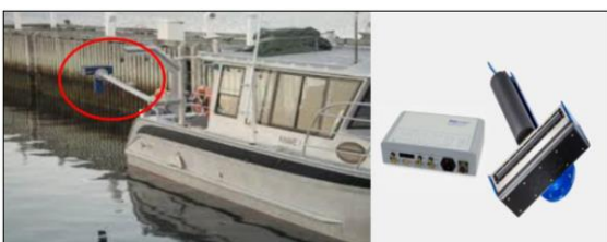
Figure 2.4 MBES R2Sonic 2024 typical configuration and equipment
