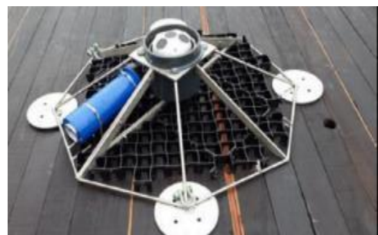
Figure 2.9 Typical seabed frame with ADCP (Ocean Scientific International Ltd)
