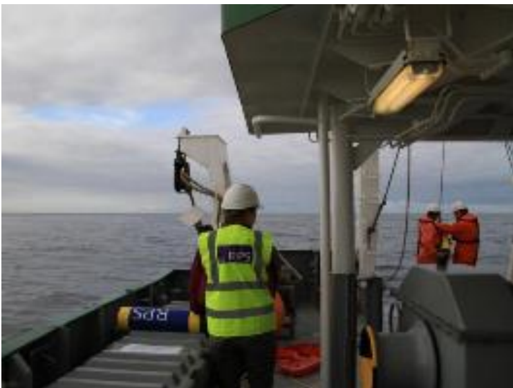
Figure 2.11 Deployment of static underwater acoustic recorders
