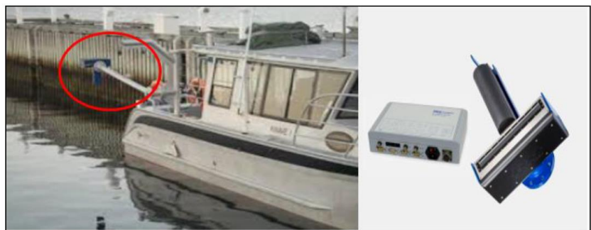
Figure 2.4 MBES R2Sonic 2024 typical configuration and equipment IMO 915882)
