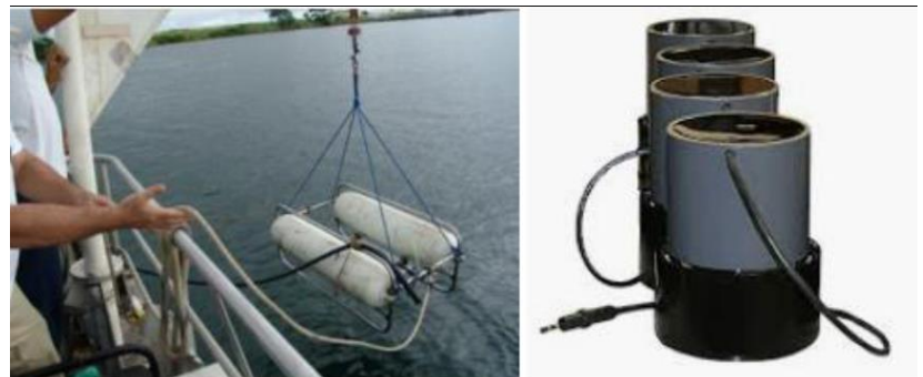
Figure 2.6 Left - Applied Acoustics AA300 being deployed & Right - Typical Hull Mounted SBP - Edgetech 3300
