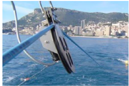
Figure 2.5 Counting pulley for winch-towed C-Max CM2 SSS
