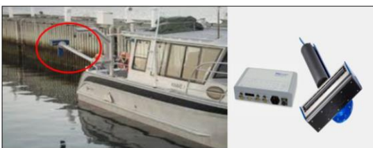
Figure 2.4 MBES R2Sonic 2024 typical configuration and equipment
