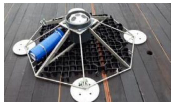
Figure 2.9 Typical seabed frame with ADCP (Ocean Scientific International Ltd)
