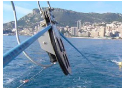
Figure 2.5 Counting pulley for winch-towed C-Max CM2 SSS
