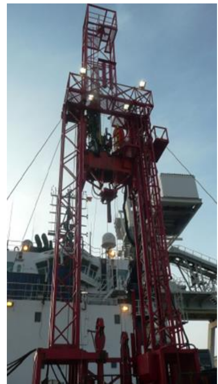
Figure 2.12 Typical marine drill (Fugro)
