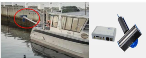
Figure 2.4 MBES R2Sonic 2024 typical configuration and equipment
