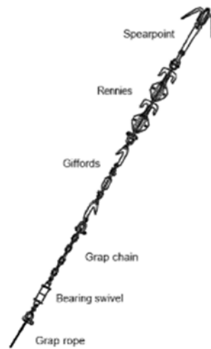
Figure 8: Typical PLGR rigging (Source: ASN, 2021)
