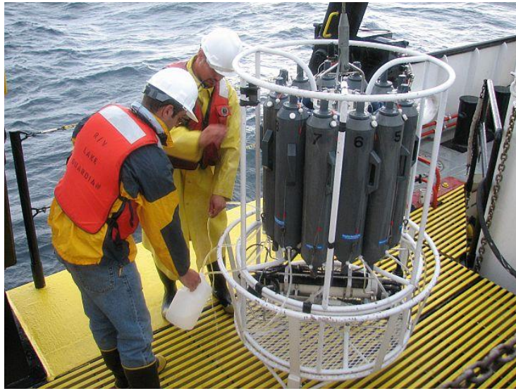
Figure 0-24: Example of CTD and Rosette sampling
