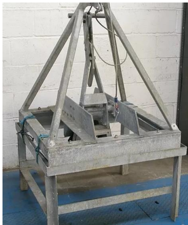
Figure 0-18: Hamon Grab (CMS – Geotech Ltd)
