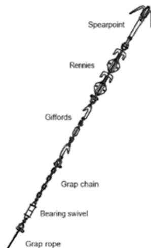
Figure 8: Typical PLGR rigging (Source: ASN, 2021)
