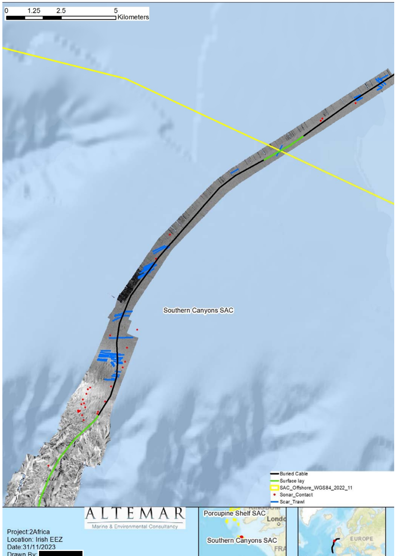
Figure 7.9. Sidescan, trawl marks (blue) and sonar contacts (e.g. boulder) in the Southern Canyons SAC.
