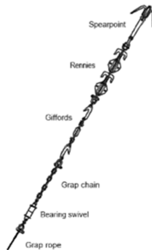
Figure 2.8: Typical PLGR rigging (Source: ASN, 2021)
